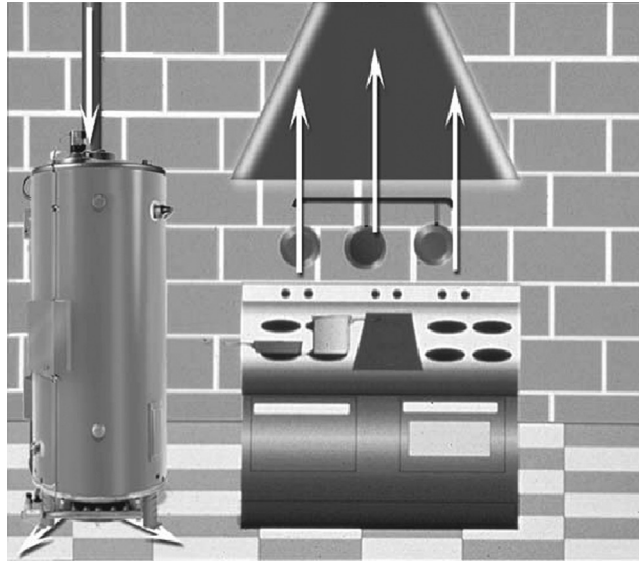
Figure 2. Downdraft Caused by Kitchen Vent Hood
